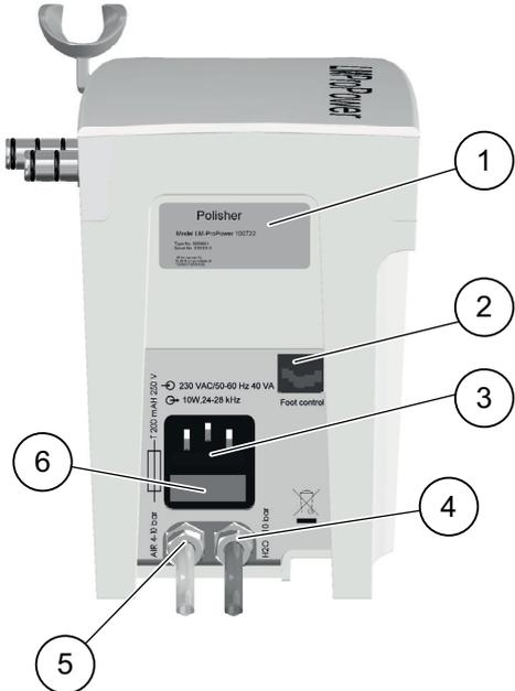
The diagram shows the rear panel of the AirLED polisher. It features a 'Polisher' label with technical specifications: 'Model: LED Polisher 10272', 'Type: 2000', 'Power: 10W', and 'Voltage: 230V'. Below this, it lists '230 VAC/50-60 Hz 40 VA' and '10W/24-28 kHz'. There are two air hose couplings labeled 'AIR 4-10 bar' and '1/2" 10 bar'. A 'Foot control' is also indicated. A fuse holder is located near the power input.
