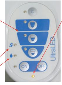
The unit is **standby** when the power cord is connected and the green LED is illuminated.
