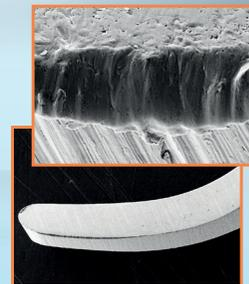
Cutting edge of an typical non-coated curette and the magnification of the edge after the test.
