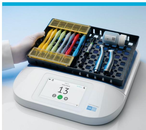
Instruments are uniquely identified with a GS1 Global Trade Item Number and serial number—identification data that is encoded as a so-called Serialised Global Trade Item Number (SGTIN) - in an EPC/RFID tag and can be read via wireless ultra high frequency (UHF) readers.
