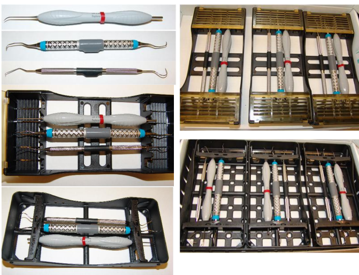
Fig 1. Dental hand instruments used in the study. On the left: instrument 1 - LM 3 ES Explorer + silicone o-ring (up); instrument 2 - Hu-Friedy Explorer EXD51, shank 31 + LM retro tagging with silicon sleeve (middle); instrument 3 - Hu-Friedy Explorer EXD5, shank with 5 mm diameter + LM retro tagging shrink wrap (below). On the right the two types of cassettes used; Servo 5 -cassettes and protected Servo 5E -cassettes.
